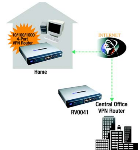
Figure 2-1: VPN Router-to-VPN Router VPN
